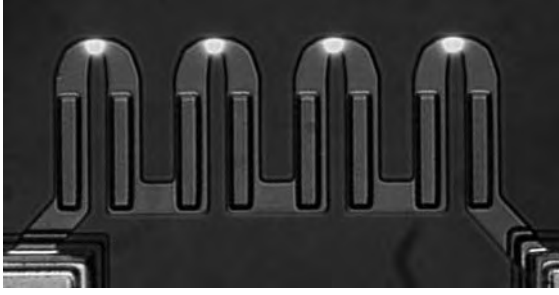
Figure 3.26 Array of four microheaters powered from a two-point connection. Hot spots show radiation. Their intensity and color code suggest equal temperatures at the hot spots.
