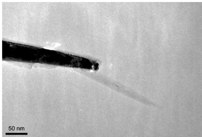
Figure 7.9 Mounted CNT tip (after N. de Jonge).
